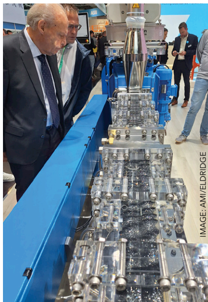
The twin screws of the new ZSK 58 Mc18 extruder were open to view at K2025
